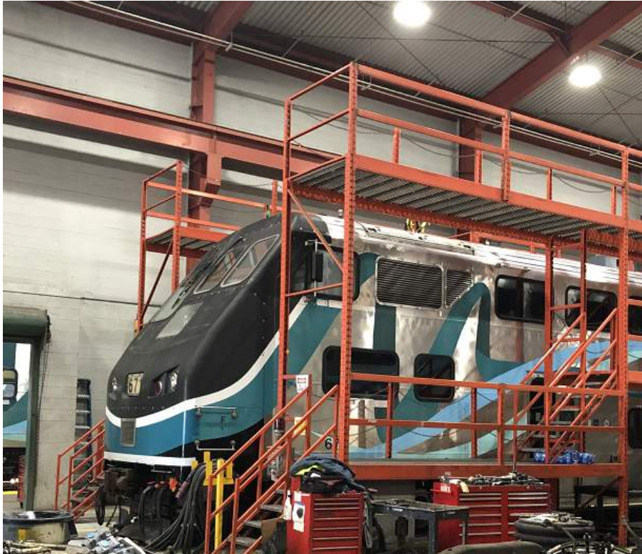
FIGURE 1-A. CAR POSITIONS WITH MULTIPLE LEVEL ACCESS
